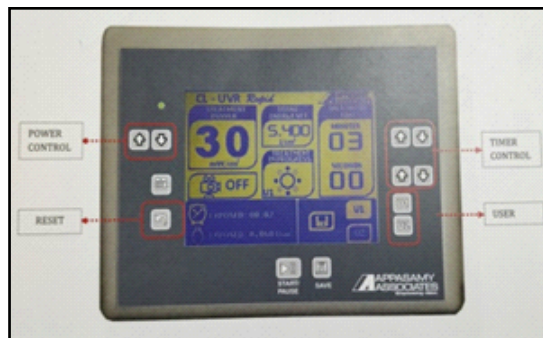
Fig.12 : CL-UVR rapid control panel menu description
